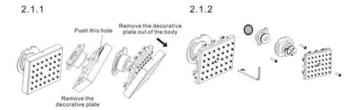
Remove the M4X12 screw and the outlet face Remove the M4X20 screw and the connector body
