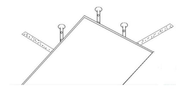
User can install can install them outside ceiling, also can concealed fixing arms in ceiling
