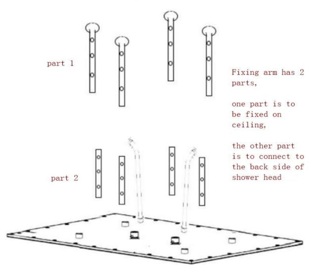
Step 3: According above step 2, connect two parts of fixing arms from shower head to ceiling. The length of the ceiling shower arms, can be adjusted from 10.2inch to 16.1inch, When decide the length of shower arm, please use screws to tighen and fix the shower arms
