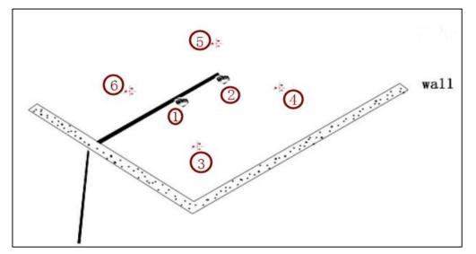
In above picture,"1" and "2" are for rainfall water inlets, to connect water hoses "3" ,"4", "5", "6" are for fixing ceiling arms
