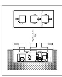
When the arrow point to 38 mark, Push the handle and turn anti-clockwise, till the arrow point to 45 mark, the temperature will attain to 45° C.and anti-process the temperature can be decreased (see figs).
