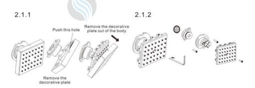
Remove the M4X12 screw and the outlet face Remove the M4X20 screw and the connector body
