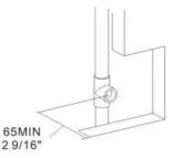
Notice: The distance between the water supply system and the finished wall be at least 65 mm.
